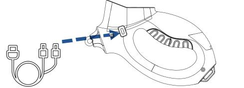
The USB charging port for the control handle can be found on the side as indicated in the photo.
